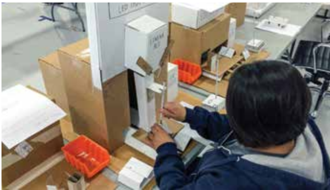
Figure 11. Process simulation and time studies for an adhesive bonding process
