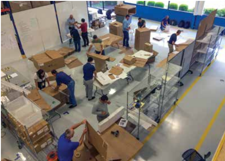
Figure 9. Constructing a 3P mockup
